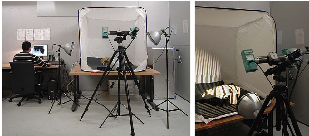
Fig. 1. (left) The setup for using the scanner: the technician controls the scanner, lamps and rotation table from the computer; (right) structured light scanner on tripod in preparation for scanning a horse skull on the rotation table.
