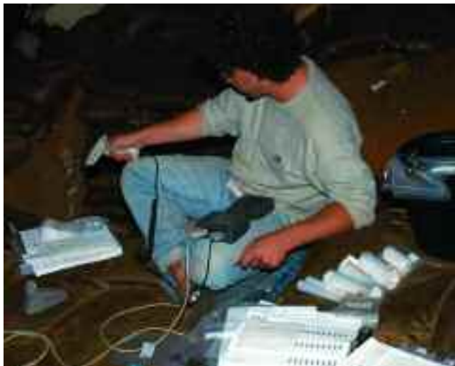
Figure 5: The Recorder with the Ranger handheld computer and the barcode scanner, scanning a Plotted Find and Lot Number to Survey Pro on the Ranger, thus linking the find to its x-y-z coordinates and stratigraphic provenience.
