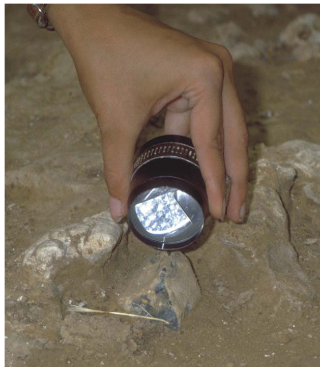
Fig. 1. The location and orientation of an artifact is measured when a total station is pointed at a prism, mounted on a short nail, held over one end of the object.
