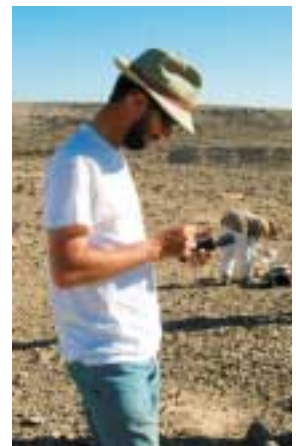
Figure 1: Using a Compaq iPAQ as a GPS in the field. The iPAQ is protected by the expansion pack in which it rests. The GPS unit is the small rectangular piece attached to the top of the unit. ESRI's ArcPad software running on Windows CE was used to record GPS points and to view our GIS layers in the field.
