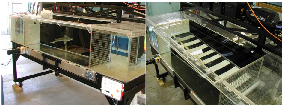
Fig. 1. Photographs of a juvenile green sturgeon subject in the apparatus built for experiments (left), showing the diffuser screen and experimental chamber; and the physical setup for Condition Below (right), where the striped optomotor belt is placed below the experimental chamber. In Condition Above, the optomotor belt is moved to the top side of the experimental chamber.
