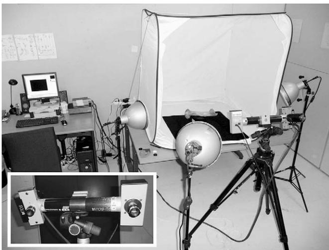
**Fig. 1.** The Breuckmann triTOS-HE structured light scanner setup in a lab with controlled lighting. The inset shows the front face of the scanner with the projector on the left and the camera on the right. The bone inside the light tent is resting on a turntable controlled by the computer. This scanner communicates with the computer via an external control (the black box sitting next to the computer) (photo by SPM).
