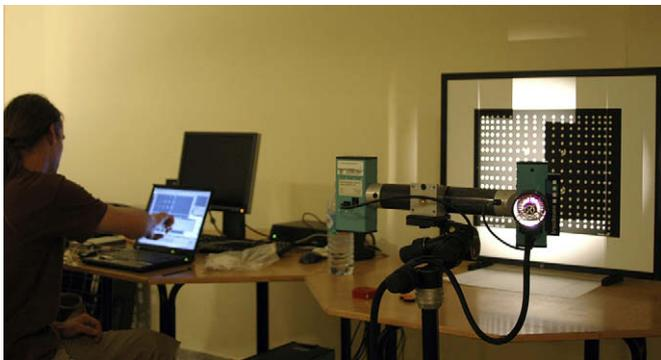
Fig. 5. Calibrating the scanner. The scanner is in the foreground on the right. It is projecting a structured light pattern on the calibration plate which is set at a fixed distance and angle from the instrument (note paper guide under the calibration plate). The calibration process is controlled by the software running on the laptop shown on the left (photo by Steffen Latsch).
